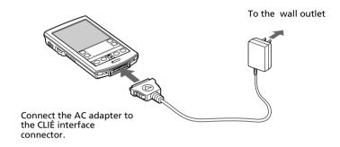
When the AC adapter is connected to your CLIÉ handheld, charging starts automatically and the battery icon on the screen changes to the battery charging icon ( ).
