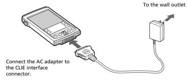
When the AC adapter is connected to your CLIE handheld, charging starts automatically and the battery icon on the screen changes to the battery charging icon ( ).
