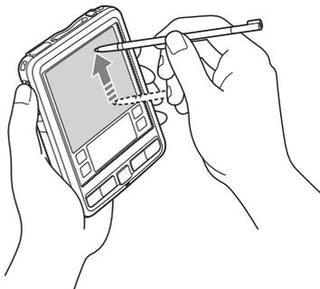
Just as you can drag the mouse to select (and drag) text or move objects on your computer, you can use the stylus to drag an item on the screen of your CLIÉ handheld. Press the stylus lightly on the item, and move it along the screen surface.
