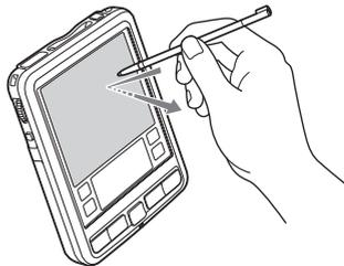
The action of pressing lightly on the screen with the stylus is called “tapping.”
