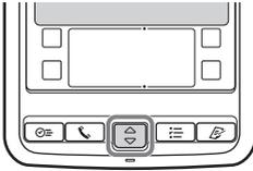
You can display text and other information that extends beyond the display area. Pushing the ▼ button scrolls down to display information below the current viewing area, and pushing the ▲ button scrolls up to display the information above the current viewing area. Depending on the application, unique features are assigned.
