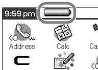
This icon indicates the remaining battery power of your CLIÉ handheld. When you tap the icon, it displays the remaining battery power of your CLIÉ handheld as a percentage, and free memory space in your CLIÉ handheld or “Memory Stick” media. When you use the outboard power, the
