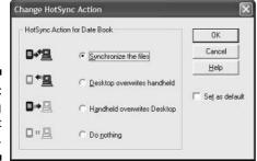
Figure 3-10: Adjusting conduit settings.
