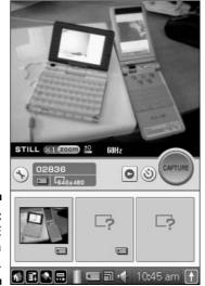
Figure 8-4: The CLIÉ Camera interface. To the right of Still is the Zoom control. The best advice here is to pretend that it doesn't exist. The CLIÉ features a digital zoom, which simulates zooming by doubling the size of the pixels in the center of the screen. That means the already-low-resolution image is going to get extremely blocky at 2X zoom and is going to turn into a fuzzy mess at 3X zoom.
