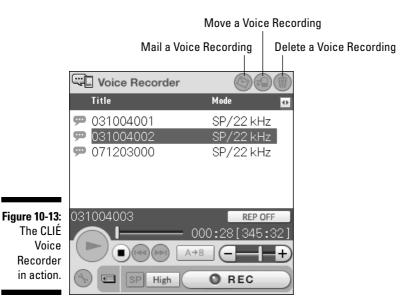
Tapping the SP/LP button to toggle between standard-play (SP) and long-play (LP) recording modes. LP mode reduces audio quality noticeably but triples the available recording time. You can use the Low/High button to set recording sensitivity. If the person speaking is near the microphone, set it to Low. If the speaker is farther away (or is what Kramer from *Seinfeld* called a *low talker*), set it to High.
