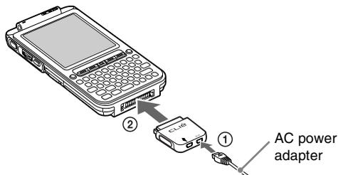
Secondly, connect the AC cord to the AC power adapter, then plug it into the wall outlet.
